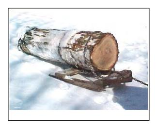
towing chain was 22% of the team's body Elevating the hitch end of the log on a go-devil reduced ground contact, friction, and motion resistance. An average draft was 724 lbf, a 14% reduction compared to using the tongs. Draft as tension in the towing chain was 49% of the weight of the load, an effort equal to 19% of the body weight of the team.
