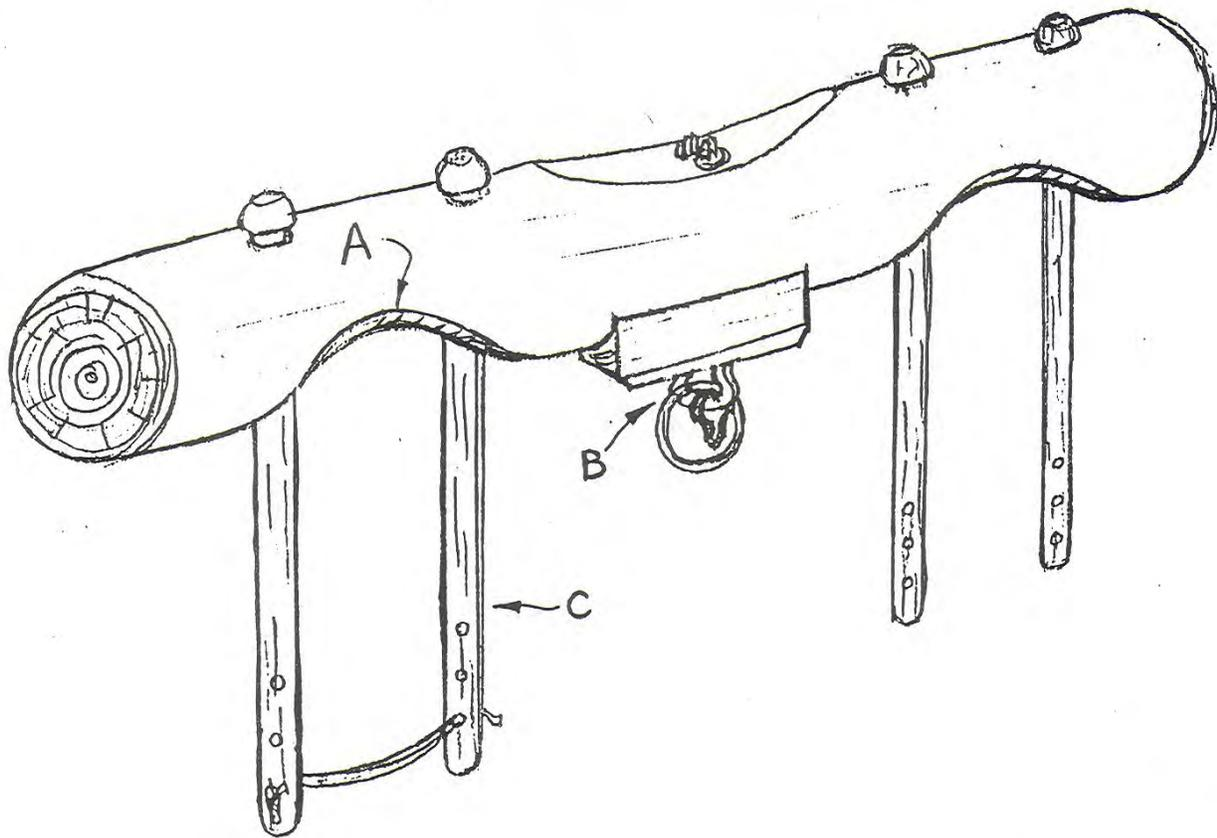
Fig. 19: One possible version of an improved yoke with a) carved neck seats b) dropped hitch point below the beam, and c) smooth round wooden staves positioned to fit the oxen's necks.
