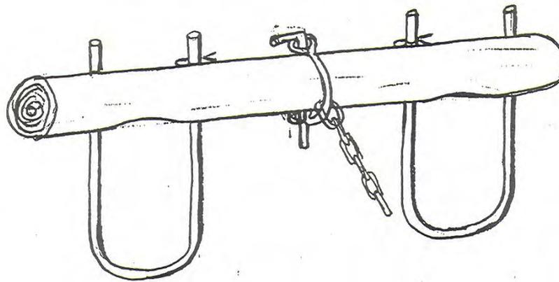
*Fig. 1: Examples of some neck yokes we have seen made from small poles in Africa. The hitch point for the chain is behind the beam. There is little or no carving to fit the neck of the oxen. Rectangular paddles or thin steel bars are used to hold the animals in position.*
