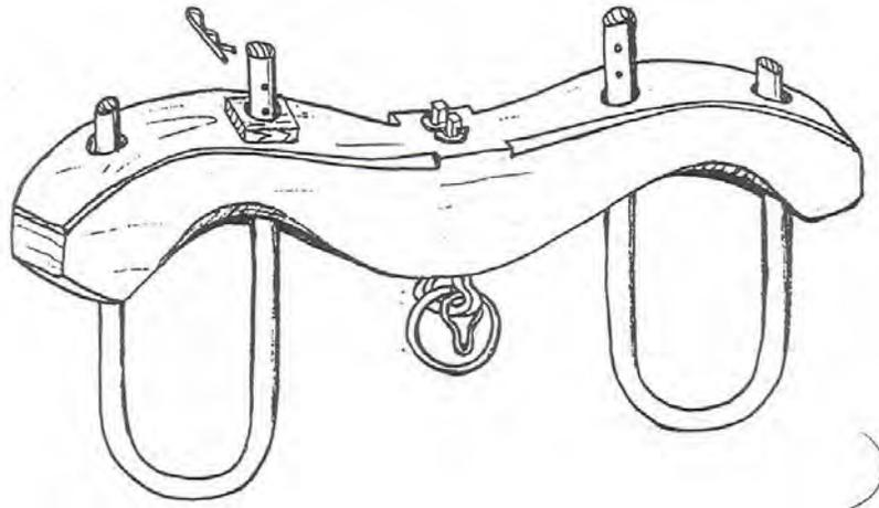
*Fig. 2: Examples of a historical neck yoke used in North American. A large beam of wood is used to construct the yoke. The beam is carved to fit over the neck of the oxen. The hitching point is below the beam. Bent wooden bows keep the oxen in position and provide an additional area for the animals to push against.*
