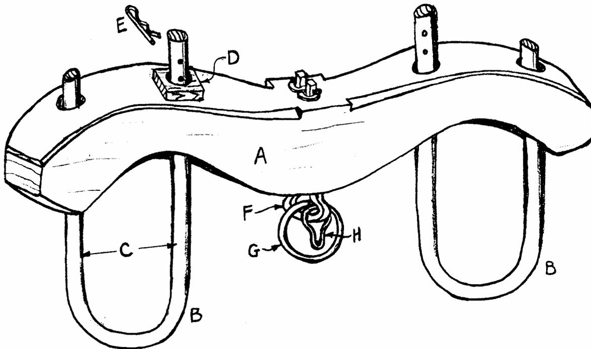
*Figure 3: Parts of a traditional neck yoke: A – yoke beam; B – bows; C – bow width and size of yoke; D – spacer block; E – bow pin; F – staple; G – pole ring; H – chain hook.*
