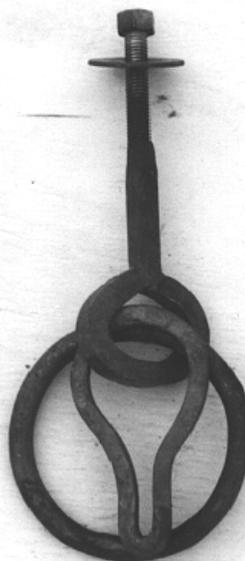
**Figure 36:** For small yokes a staple with a single threaded stem and a closed bulb works well.
