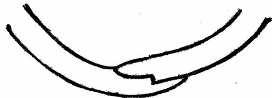
**Figure 28:** The lap pattern for a scarf weld on the rings.
