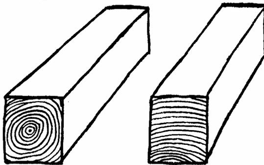
**Figure 7:** A beam with the grain pattern shown on the right is a better choice for yoke making.
