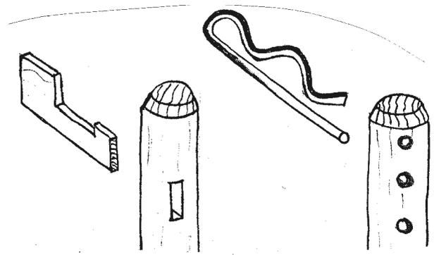
*Figure 24: Wood or metal bow pins keep the bow in the yoke beam.*
