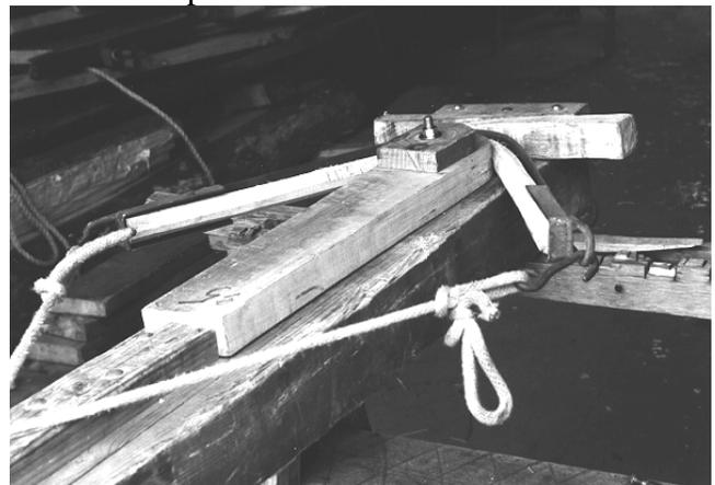
**Figure 21: bending a bow on the jig.**
