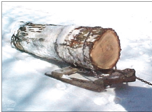
A go-devil elevates the hitch end of the log.
