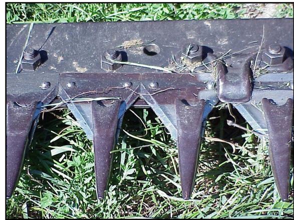
Guards protect the knives from impact damage, guide the crop into the knives and hold a stationary ledger plate.
