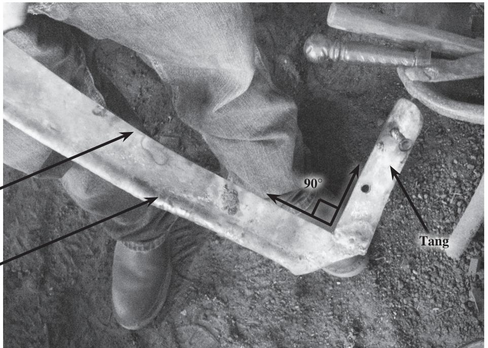
Pin, bent at 90 degrees to the flat of the rest of the blade.
