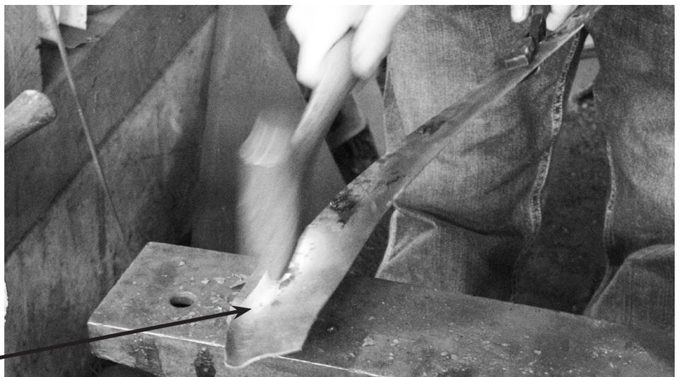
Use a straight pein to hammer the outside edge into a swedge block or groove, forming a bend along the full length of the blade.
