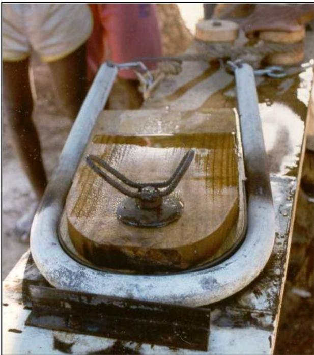
Fig. 15: Bending metal pipes to make ox bows.
