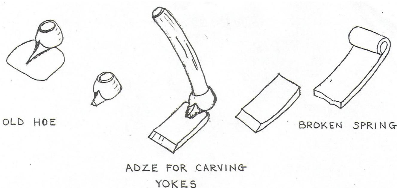
*Fig. 13: A blacksmith can make an adze from an old hoe and a spring from a truck.*
