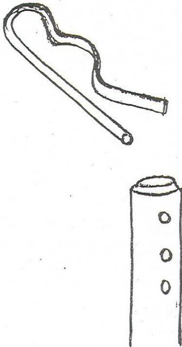
*Fig 17: A pin to hold the bow can be made from the spring of a broken bicycle seat.*
